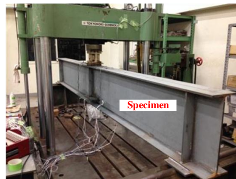
Photo 1. Loading test set up.
