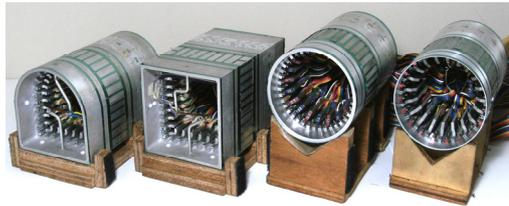
Arch-type Box-type Rigid-pipe Flexible-pipe
