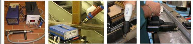
Fig. 9: Examples of four different tools for high frequency peening treatment. M.M. Pedersen, et al.: Comparison of Post Weld Treatment of High Strength Steel Welded Joints in Medium Cycle Fatigue, XIII-2272-09, IIW引用
